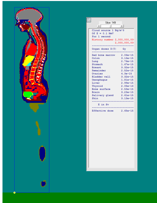
Figure 17. Female ICRP phantom exposed to 1 \text{ Bq/m}^3 of photons of 100 keV for one second. The white lines in the air indicate the start point and initial direction of the photons emitted.
